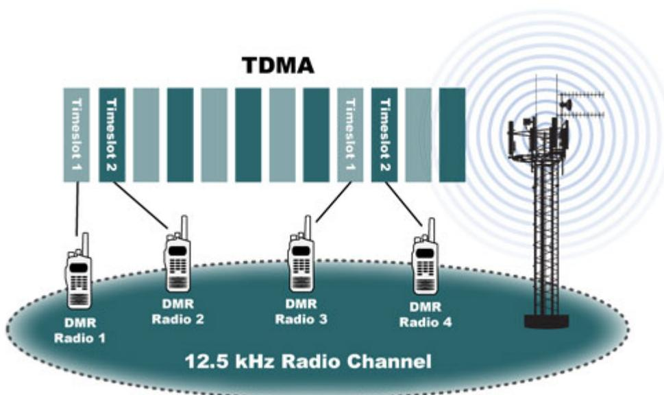
In this arrangement each communication path is active for half of the time in 12.5 kHz of bandwidth and so each uses an equivalent bandwidth of half x 12.5 kHz or 6.25 kHz . This is known as having an efficiency of one talk path per 6.25 kHz of spectrum, but with DMR the channel as a whole maintains the same profile as an analogue 12.5 kHz signal.
