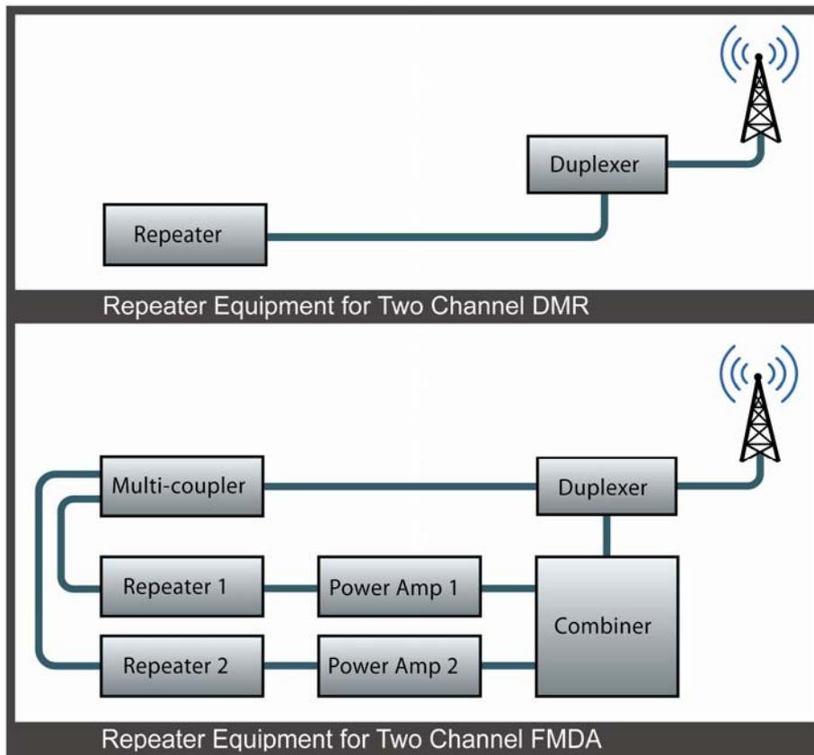
FDMA requires a dedicated repeater for each channel, plus expensive combining equipment to enable multiple frequencies to share a single base-station antenna. It can be particularly expensive to make combining equipment work with 6.25 kHz signals, and there's typically a loss in signal quality and range when it's used in this way, hence the need for power amplifiers shown in diagram 6.
